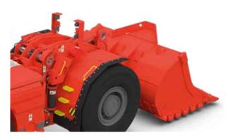
Improved boom locking mechanism enables one-handed operation and maintaining 3-point contact. The boom uses lighter hollow pins which are easier to remove, along with new bush lip sealings to prevent the ingress of dirt, reducing wear. Sandvik LH621i is equipped with more greasing points in the boom geometry, well protected grease lines and automatic central lubrication system with increased capacity for longer time between refilling.
