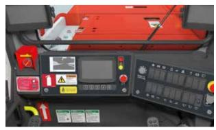
To minimize the need to move around the machine or use special tools, the 7" colour display in the operator's compartment provides service information, easy system diagnostics and alarm log files.
