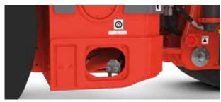
The cold side includes a filter station for engine and brake filters with ground level access. An efficient Power Core engine filter is housed well within the frame, and it utilizes an ejector valve system for increased filter lifetime.
