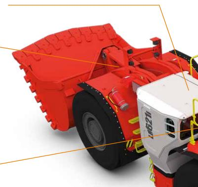
Separate battery and starter isolation switches are located at ground level access for troubleshooting while the engine is locked out for service.
