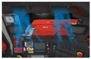
keep eyes on the road. New, darker background graphics with clearer symbols have been designed to reduce eye fatigue in the underground mining environment.
